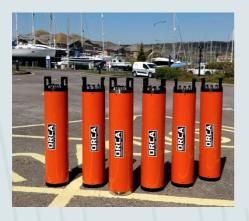
*Orca* is a broadband underwater acoustic recorder that supports multiple hydrophone channels and extremely high sampling rates.
