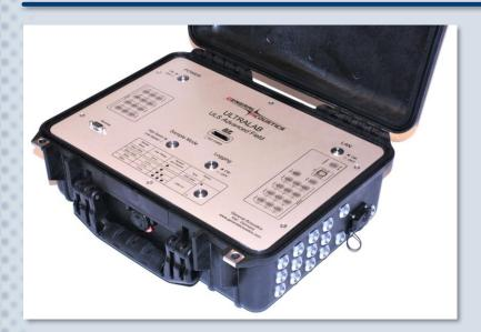
A 4-channel UltraLab Advanced Field controller in its rugged Peli-Case, fit for numerous demanding wave measurement applications outdoor, offshore, in the field.
