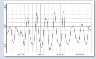
Two exemplary results showing different wave situations evaluated with an UltraLab Advanced field. A ship-induced wave at river Elbe, is shown on the left. The right plot shows a wave field captured at the north sea. The wave height in meters is plotted over time.
