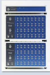
PTP-Synchronization enables the connection of multiple controllers to perform fully synchronized. PTP-Client and Grandmaster are utilized to connect two UltraLab HF units here.
