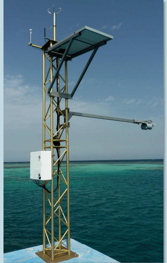
A LOG_aLevel station with a long range ultrasonic sensor, reference track and additional meteorological sensor, located at Red Sea. This unit is solely powered by a vertical solar panel.
